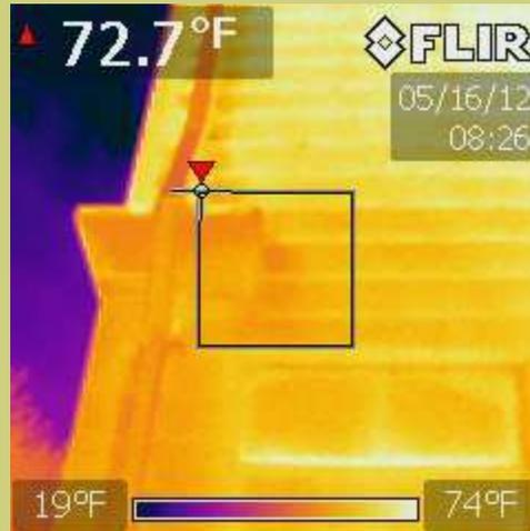
Figure 4. Leak behind siding.
