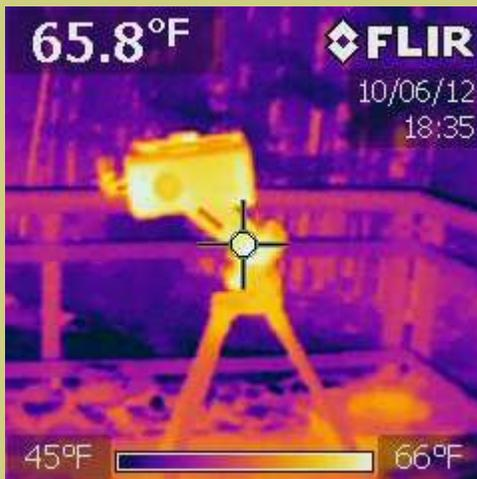
Figure 7. Telescope before cooling.
