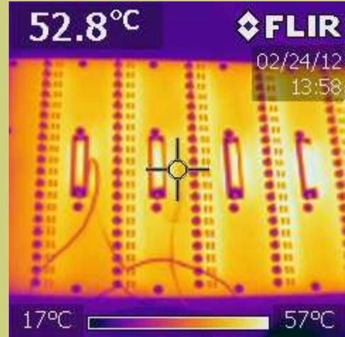
Figures 5, 6. Thermal image of a circuit board.
