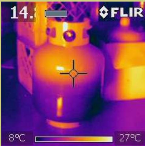
Figure 9. Propane cylinder fuel level.
