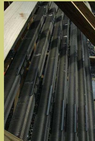
Figures 1, 2. Heat Dump (baseboard radiant tubing).
